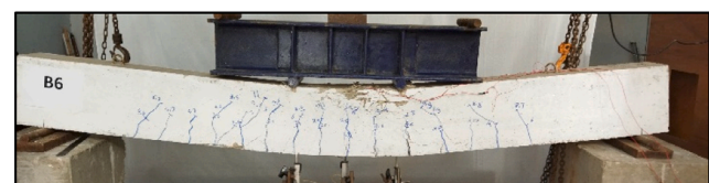
(f) Crack Patterns for the Tested Beam B6
