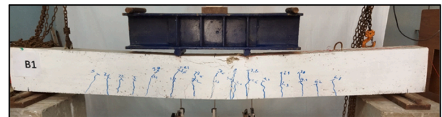
(a) Crack Patterns for the Tested Beam B1
